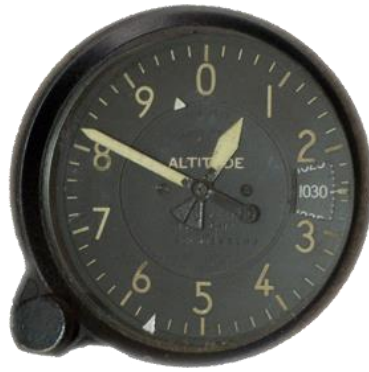
Fig 2. With QNH set in the sub-scale, altimeter reads altitude
