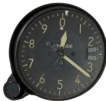
Fig 1. With standard pressure 1013 set in the sub-scale window an altimeter reads pressure height
