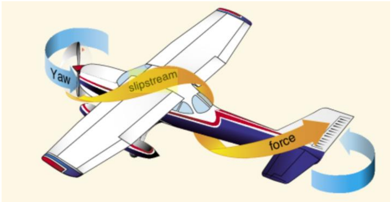
Fig 2-23: Corkscrew Effect of Slipstream.
