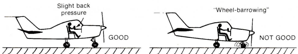
Fig 12.9: Protect the Nose Wheel
